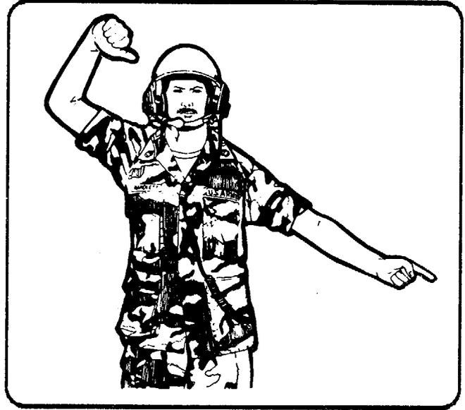
The signal to **LOWER THE SPADE** is made in the same way, but with the thumb of the right hand pointing downward.
